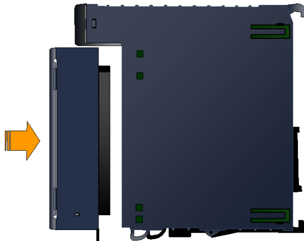
Figure 429: Installing a High-Density Terminal Block
