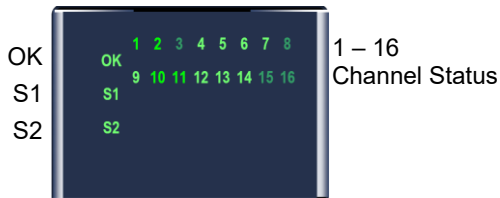
Figure 217: LED Layout MDL765
