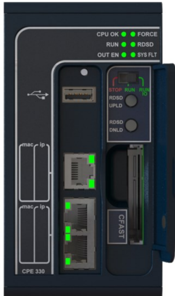
Figure 47: CPE330 (example of 2-Slot CPU)
