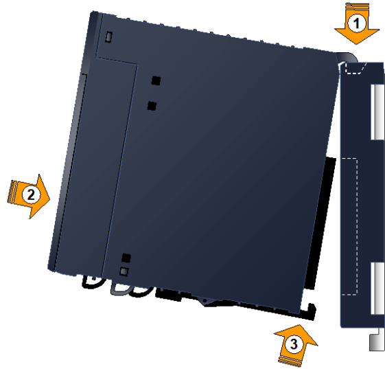
Figure 24: Installing The module in Backplane
